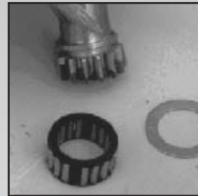
Clean all parts with solvent except 37848/37849.
