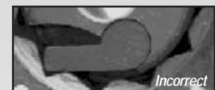
If ratchet gear is mounted backwards, winch will slip.
