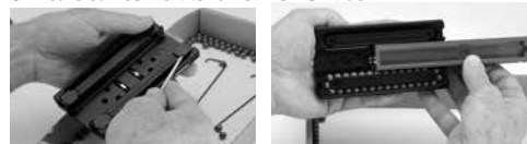
Remove corner keepers and retaining clips and load balls using car loader.
