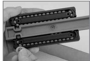
6. Put one (1) clip on "open" end of loader. Load rest of balls through ball loading port into empty bearing race. Consult chart to confirm quantity. Line up car loader with track and gently roll car onto track.
