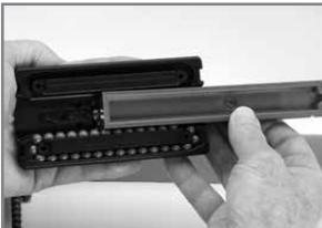
5. Remove two (2) clips from car loader. Slide car loader in so loading port is on the side of car without balls.
