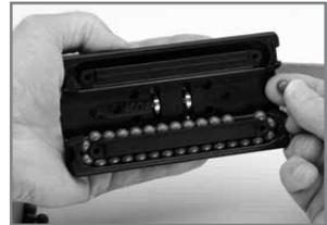
4. Hold car on edge and load lower side with correct number of balls. **DO NOT OVERLOAD.** Consult chart to confirm quantity.
