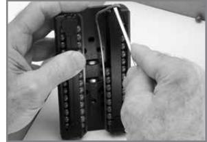
2. Pry retaining clip off and dump balls in box.
