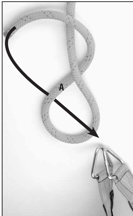
Come up from underneath "A" to make a figure 8.
