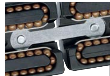
Recessed stainless steel car coupler adjusts to fit curved track
